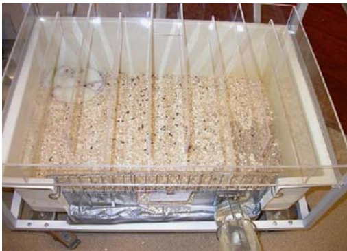
Figure 2. Second floor (maze) constructed of Plexiglas.
